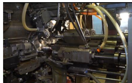
Figure 2: internal view of the multi-spin cam lathe
