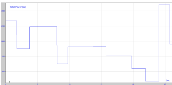
Fig. 4. Energy consumption of the molding station throughout the process, collected via SMS.
